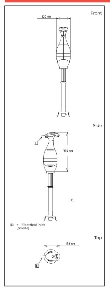
Electric Supply voltage: 220-240 V/1 ph/50/60 Hz **Electrical power max.:** 0.45 kW 0.45 kW **Total Watts:** Capacity: Capacity (up to): 80 Litre Key Information: External dimensions, Width: 138 mm External dimensions, 120 mm Depth: External dimensions, Height: 665 mm **Shipping weight:** 4.2 kg
